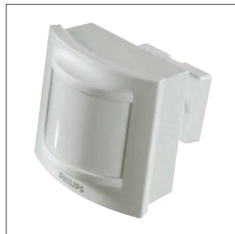
High-bay passive infrared movement detector (mounting height up to 15 m), equipped with an adjustable delay timer (up to 35 minutes). Can be used with all MDU control units. A dedicated mounting bracket (ZTX400 MB-MDU) is available, into which the movement detector can be clicked
